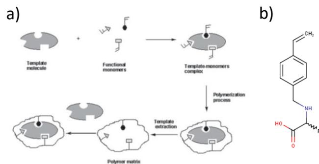
**Figure 1: a) Formation of a MIP around a template molecule. b) Target functional monomer. R designates amino-acids side-chains.**
